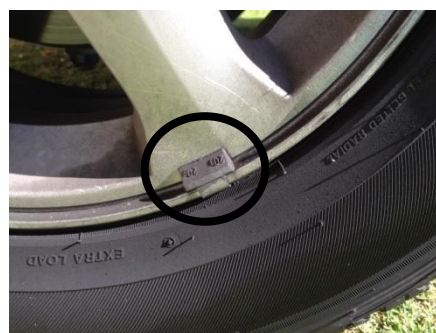
Diagrams of a car wheel with a wheel weight clipped on to the rim.
